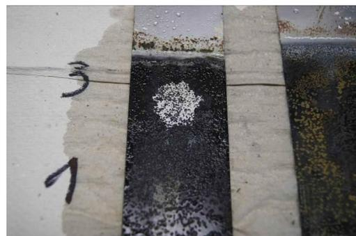
Vinkocide SR 3 shows an excellent removal of the biofilm. It also removes corrosion products.
