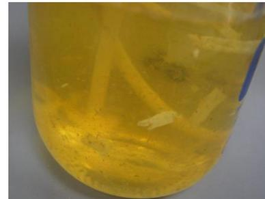
The efficacy of Vinkocide SR 3 + DBNPA can be characterized by the destruction of the EPM and of the cell structures. Dead biomass is produced and largely discharged. The removal of biofilms is better from metal surfaces than from plastics.
